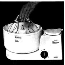
If light dough is to be kneaded or foam substance is to be beaten, set the beaters on the shaft of the mixing bowl. When creaming butter make sure that it is at room temperature. Heavy dough or hard butter can damage the beaters. For heavy dough use the kneading arm from start to finish.
